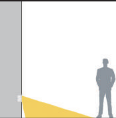
偏配光设计，适用于人行步道及广场 Asymmetric beam angle improved visual comfort to the pedestrian
